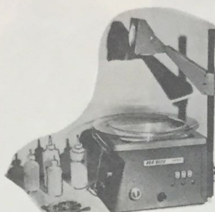
"Travelgraph" overhead projector set up for wet show. Non-mixing colored liquids (oil, water) are pooled into larger dish, then smaller convex dish is "splashed" into the colors in bottom dish. Dyes are stored in plastic bottles.
